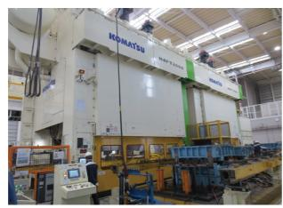
3500-ton servo module transfer press
